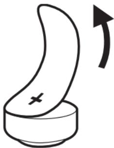
Take the adhesive tab off the new battery and make sure there is no sticky substance left on it. Let it "breathe" for 60 seconds.
